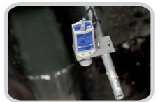
The Cello CSO Level recorder has sophisticated alarm regimes for detecting and immediately signalling abnormal conditions. These include high & low alarms levels as well as profile alarms. The Cello also reports in-situ signal strength, GSM network errors and low battery levels
